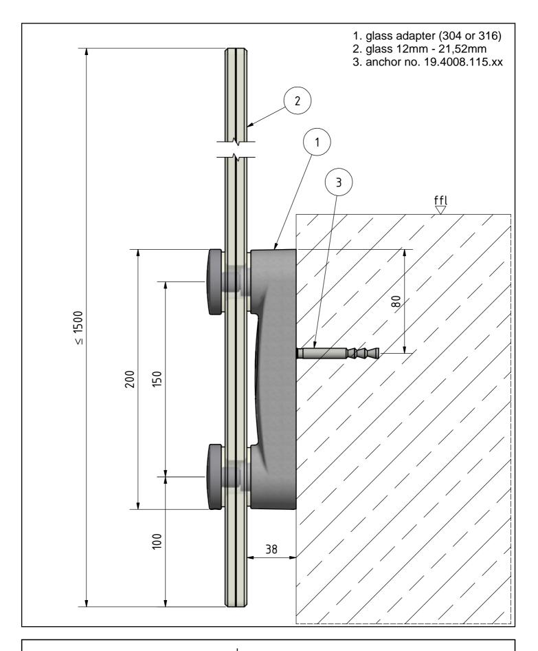
SYSTEM:Easy GlassMODEL:0762DESCRIPTION:Glass adapterDRAWN:TRRDATE:06.04.2020DRAWING NO.:0762-001
